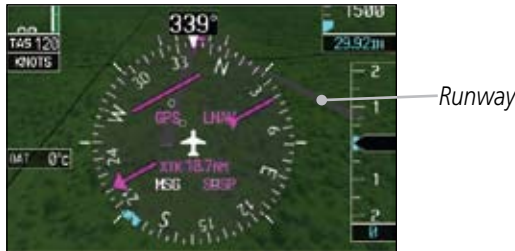
Figure 5-40 Depiction of Runway Not in Loaded Flightplan
